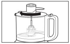
Install the Work Bowl cover, making sure the Lid Latch is pushed down to the locked position.
