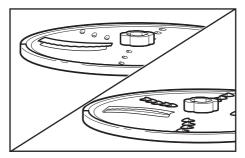
The disc can be placed in two different positions: high at the top of the bowl for processing, and low in the bowl for storage.
