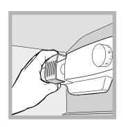
Access the light bulb by removing the cover as indicated in the diagram. Replace it with a similar light bulb within the power range indicated on the cover (15W or 25W).
