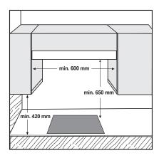
NOTE: Kitchen cabinets adjacent to the appliance and taller than the top of the hob must be at least 200 mm from the edge of the hob. Hoods must be installed according to their relative installation instruction manuals and at a minimum distance of 650 mm from the hob (see figure). Place the wall cabinets adjacent to the hood at a minimum height of 420 mm from the hob (see figure). If the hob is installed beneath a wall cabinet, the latter must be situated at a minimum of 700 mm above the hob.
