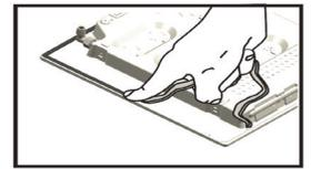
To secure the hob, use the brackets (A) provided with it. Fit the brackets into the relevant bores shown by the arrow and fasten them by means of their screws in accordance with the thickness of the worktop (see the following figures).
