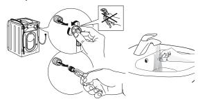
**4.** Insert the mesh filter again. Connect the inlet hose to water tap and washing machine again. Do not use a tool to connect the inlet hose. Open the water tap and check that all connections are tight.
