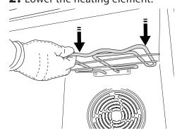
**3.** To return the heating element to its position, lift it up, pull it slightly towards you and make sure that the tab support is in its proper seating.
