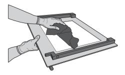
**3.** To correctly reposition the inner glass, make sure that the "R" is visible in the right-hand corner and the clear surface (not printed) is facing up. First insert the long side of the glass indicated by "R" into the support seats, then lower it into position.
