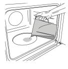
Only when the oven is cold, fill the embossing of the cavity with the quantity of drinking water suggested in the relative cooking table.
