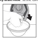
5. Turn the stopper of the "emergency drain hose" at the end of the hose and let the water flow into the container.
