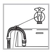
Alternatively, place the drain hose over the edge of a washbasin or bathtub, by fastening the guide (which can be purchased at the technical assistance centre) to the tap (see figure). The free end of the
