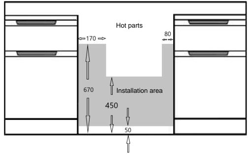
Position the gas connection point such that it is located within the shaded area, and the hose also hangs naturally within the shaded area.
