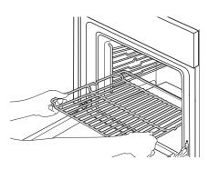
Other accessories, such as the drip tray and the baking tray, are inserted horizontally in the same way as the wire shelf.
