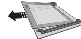
3 To correctly reposition the inner glass, make sure that the "R" is visible in the left-hand corner and the clear surface (not printed) is facing up. First insert the long side of the glass indicated by "R" into the support seats, then lower it into position (4). Refit the upper edge (5): a click will indicate correct positioning. Make sure the seal is secure before refitting the door.
