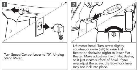
**NOTE:** When properly adjusted, the Flat Beater will not strike on the bottom or side of the Bowl. If the Flat Beater or the Wire Whip is so close that it strikes the bottom of the Bowl, coating may wear off the beater or wires on whip may wear.
