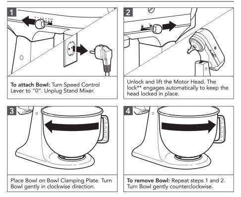
**NOTE:** Motor Head should always be in locked position when using the Stand Mixer. \*Included with select models only. Also available as optional accessory. \*\*Locking option is available on select models.
