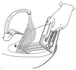
Clean the filter chamber of the dryer with a damp cloth or carefully with a vacuum cleaner. Insert the bottom filter again. Turn the locking bars upwards in vertical position. Close the bottom flap.
