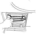
Clean the bottom filter under running water; wipe away dust and
