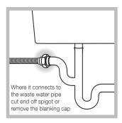
The drain hose may be connected to an under-sink trap. Before connecting the drain hose from the machine ensure that any blanks or removable ends have been taken off the spigot.
