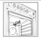
2. Unscrew the grill burner nozzle using a special nozzle socket spanner (see figure) or preferably with a 7 mm socket spanner, and replace it with a new nozzle that is suited to the new type of gas (see Burner and nozzle specifications table
