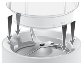
4. Press down and rotate Culinary Blender Jar clockwise, approximately 1/4 turn through two steps of resistance (until two clicks are heard).
