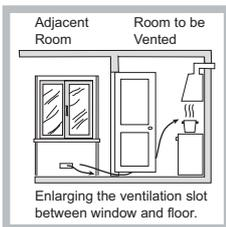
The system can also provide the air needed for combustion indirectly, i.e. from adjacent rooms fitted with air circulation tubes as described above. However, these rooms must not be communal rooms, bedrooms or rooms that may present a fire hazard.
