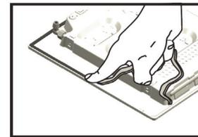
Apply the seals that come with the appliance along the outer edges of the hob to prevent any passage of air, humidity and water (see Figure). For proper application make sure the surfaces to be sealed are clean, dry and free of any grease/oil.
