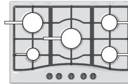
The more variable aspect in terms of pan stability can often be the pan itself, (or the positioning of that pan during use). Well balanced pans, with flat bases that are placed centrally over the burner, with the pan handles aligned with one of the support fingers obviously offer the greatest stability.
