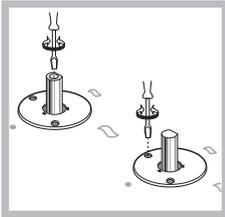
2. Remove the knob and adjust the adjustment screw, which is positioned in or next to the tap pin, until the flame is small but steady.
