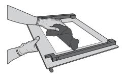
**3.** Refit the intermediate pane (marked with "R1") before refitting the inside pane: To position the panes of glass correctly, make sure that the "R" mark can be seen in the left-hand corner. First insert the long side of the glass indicated by "R" into the support seats, then lower it into position. Repeat this procedure for both panes of glass.
