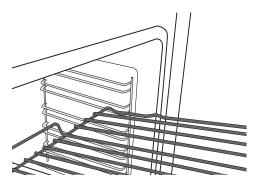
• The other accessories, such as the baking tray, are inserted horizontally in the same way as the wire shelf.
