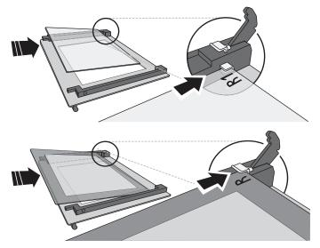
**4.** Refit the upper edge: A click will indicate correct positioning. Make sure the seal is secure before refitting the door.
