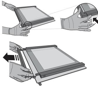
**2.** Lift and firmly hold the inner glass with both hands, remove it and place it on a soft surface before cleaning it.
