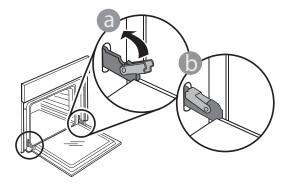
**5.** Try closing the door and check to make sure that it lines up with the control panel. If it does not, repeat the steps above: The door could become damaged if it does not work properly.
