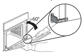
**4.** Take a firm hold of the door with both hands – do not hold it by the handle. Simply remove the door by continuing to close it while pulling it upwards at the same time until it is
