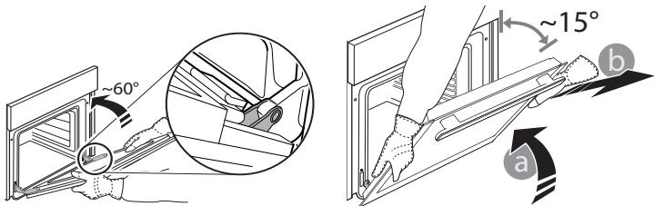
3. Refit the door by moving it towards the oven, aligning the hooks of the hinges with their seating and securing the upper part onto its seating.
