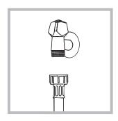
1. Connect the supply pipe by screwing it to a cold water tab using a 3/4 gas threaded connection (see figure). Before performing the connection, allow the water to run freely until it is perfectly clear.
