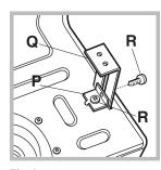
Fig. 8 Accessories provided for the height adjustment.
