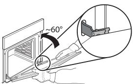
**4.** Take a firm hold of the door with both hands – do not hold it by the handle. Simply remove the door by continuing to close it while pulling it upwards at the same time until it is
