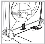
2. make sure the water level inside the machine is lower than the door opening; if it is not, remove excess water using the drain hose, collecting it in a bucket as indicated in the *figure*.
