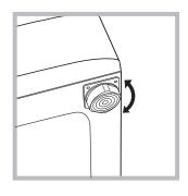
2. If the floor is not perfectly level, compensate for any unevenness by tightening or loosening the adjustable front feet (see figure); the angle of inclination, measured in relation to the worktop, must not exceed 2°.
