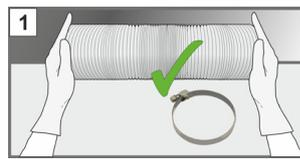
Remove 'oval-shaped' Ventilation hose from the packaging. Ensure that you also remove the jubilee clip. If you require to reduce the length of the hose please wear gloves when cutting the hose.
