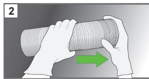
Pull to expand the end of the Ventilation hose prior to fitting. If the hose has not been expanded, the jubilee clip will not clamp the hose to the adaptor.
