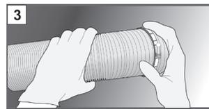
Place one of the jubilee clip over the end of the extended vent hose. An additional jubilee clip can be used to secure the opposite end of the vent hose to a wall mounting kit (kit and clip not supplied).
