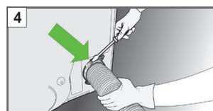
Clamp the ventilation hose to the rear vent outlet by tightening the jubilee clip with a screwdriver. If the hose has not been expanded, the clip will not clamp the hose to the rear vent outlet.
