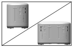
3. Press down on the Start Lever to start the toasting cycle. The toast will pop up automatically at the end of the cycle and the Toaster will turn off.
