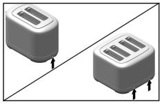
3. Once the Crumb Tray has opened slightly, slide it out of the Toaster and shake the crumbs into a waste container.
