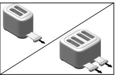
**IMPORTANT:** Be sure to open the Crumb Tray by pressing the PUSH icon. Forcing the Crumb Tray open may damage the Crumb Tray.
