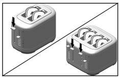
3. Press Bagel button ( (1)); the Bagel Indicator Light will glow. The bagels will pop up automatically at the end of the Cycle and the Toaster will turn off.
