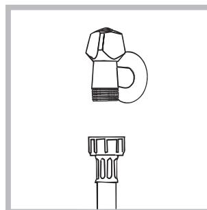
1. Connect the supply pipe by screwing it to a cold water tap using a  $\frac{3}{4}$  threaded connection (see figure). Before performing the connection, allow the water to run freely until it is perfectly clear.
