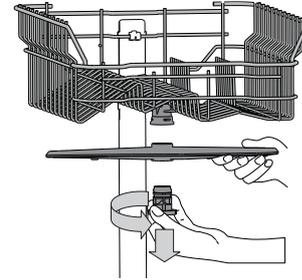
To remove the upper spray arm, turn the plastic locking ring in an anti-clockwise direction. The upper spray arm should be replaced so that the side with the greater number of holes is facing upwards.
