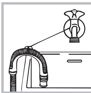
alternatively, placed it over the edge of a basin, sink or tub, fastening the duct supplied to the tap (see figure). The free end of the hose should not be underwater.
