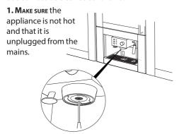
**2. Using a screwdriver,** unscrew the screw fixing the espresso boiler outlet filter.
