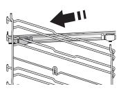
Fasten the upper clip of the runner to the shelf guide and slide it along as far as it will go. Lower the other clip into position.
