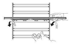
**4.** To secure the guide, press the lower portion of the clip firmly against the shelf guide. Make sure that the runners can move freely.
