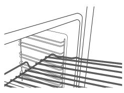
• The other accessories, such as the baking tray, are inserted horizontally in the same way as the wire
