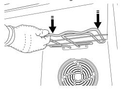
**3.** To return the heating element to its position, lift it up, pull it slightly towards you and make sure that the tab support is in its proper seating.
