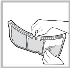
2. Clean the fluff off the filter and replace it correctly. Ensure that the filter is pushed fully home.
