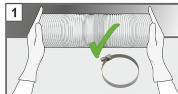
Remove oval-shaped Ventilation hose from the packaging. Ensure that you also remove the two jubilee clips. If you require to reduce the length of the hose please wear gloves when cutting the hose.
