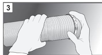
Place one of the the jubilee clips over the end of the extended vent hose. The second jubilee clip can be used to secure the opposite end of the vent hose to a wall mounting kit (not supplied).
