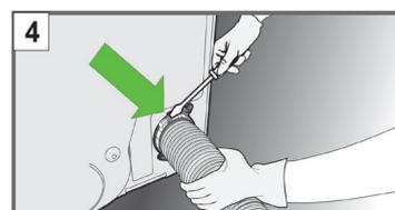
Clamp the ventilation hose to the rear vent outlet by tightening the jubilee clip with a screwdriver. If the hose has not been expanded, the clip will not clamp the hose to the rear vent outlet. The tumble dryer may protrude further forward from the worktop. Please do not push the tumble dryer too far backward.
