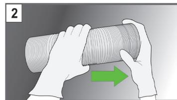
Pull to expand the end of the Ventilation hose prior to fitting. If the hose has not been expanded, the jubilee clip will not clamp the hose to the adaptor.
