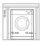
If you are going to install the appliance under a work counter be sure to leave a 10mm space between the top and any other objects on or above the machine and a 15mm space between the sides and any kitchen units or walls to ensure proper air
