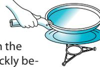
**DO NOT PLACE ANY UTENSILS** on the Crisp-plate since it will quickly become very hot and is likely to cause damage to the utensil.
