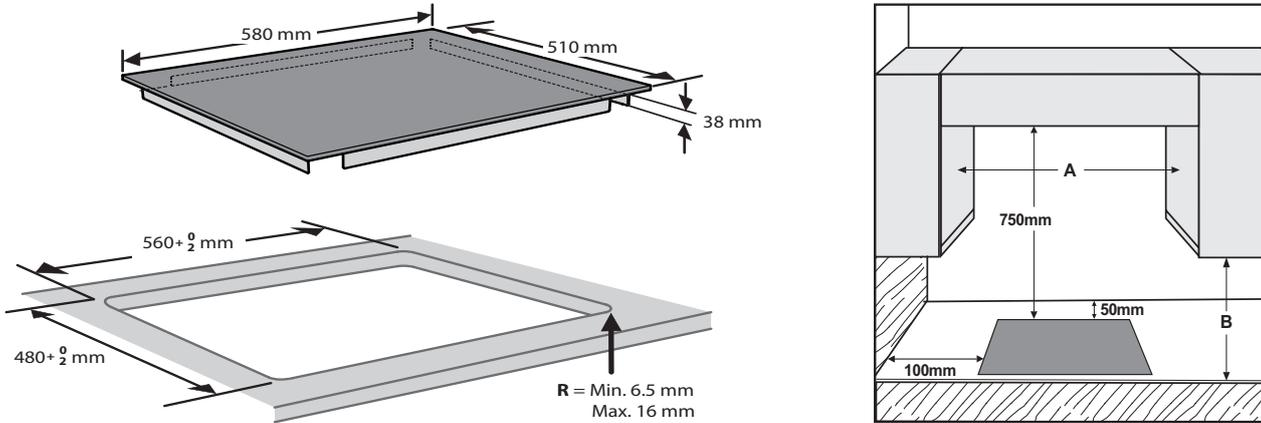
**NOTE: if distance "A" between the kitchen cabinets is between 600 mm and 730 mm, height "B" must be at least 530 mm. If distance "A" between the kitchen cabinets is greater than the width of the hob, height "B" must be at least 400 mm. If a hood is installed above the hob, refer to the assembly instructions for the hood to see the necessary distance.**
