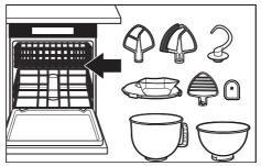
**IMPORTANT:** The Wire Whip is only dishwasher-safe for models 5KSM200, 5KSM180, 5KSM185 and 5KSM193. For all other models: Wash it thoroughly in hot sudsy water and rinse completely before drying. Do not store Wire Whip on shaft.
