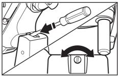
**NOTE:** When properly adjusted, the Flat Beater\* will not strike on the bottom or side of the Bowl. If the Flat Beater\* or the Wire Whip is so close that it strikes the bottom of the Bowl, coating may wear off the beater or wires on whip may wear.
