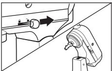
**3.** Slip accessory onto Beater Shaft and press upward as far as possible. Then, turn accessory to the right, hooking accessory over the pin on the shaft.
