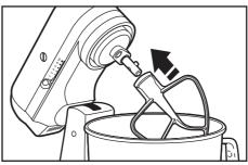
**4.** To remove accessory: Repeat steps 1 and 2. Press accessory upward as far as possible and turn to the left. Then pull accessory from the Beater Shaft.
