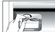
Repeat Step 2 for the other half of the tray, if necessary. To get ice, slightly lift up the storage bin and pull it towards you.
