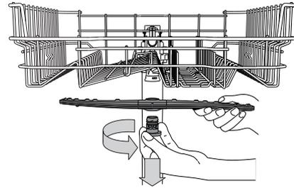
To remove the upper spray arm, turn the plastic locking ring in an anti-clockwise direction. The upper spray arm should be replaced so that the side with the greater number of holes is facing upwards.
