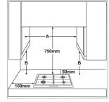
**NOTE:** If the distance "A" between the wall cabinets is between 600 mm and 730 mm, the height "B" must be a minimum of 530 mm. If the distance "A" between the wall cabinets is greater than the width of the hob, the height "B" must be a minimum of 400 mm.
