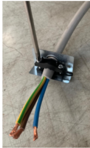
Fix power cord to the plastic holder.
