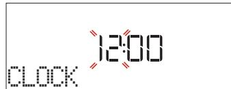
Turn the *adjustment knob* to set the current hour and press ✓: The two digits for the minutes will flash on the display. Turn the *adjustment knob* to set the minutes and press ✓ to confirm.
