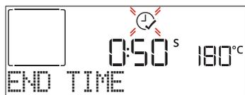
Turn the *adjustment knob* to set the time you want cooking to end, then press
