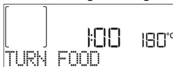
An audible signal will sound and the display shows the action to be done: Open the door, do the action prompted by the display, close the door, and resume cooking.
