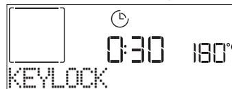
Please note: This function can also be activated during cooking. For safety reasons, the oven can be switched off at any time by turning the *selection knob* to "0".
