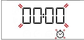
Use + or - to set the time you require and press
