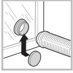
towards the air inlet pipe on the rear of the appliance. The ventilation hose must always be fitted to ensure optimum performance. Make sure that the ventilation hose and the air inlet vents are not obstructed or blocked. Do not let the tumble dryer recirculate exhaust air.
