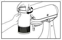
Remove the Ice Cup from the housing by rotating it to the right and pulling downward. Take note of the small indicator arrow which must line up with the Lock and Unlock symbols on the housing.
