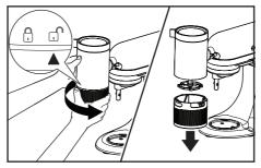
**OPTIONAL:** If you wish to change the blade, grip the blade from the bottom and rotate it to right to unlock and remove.
