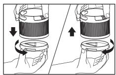
2. Each of the interlocking tabs is a unique size, ensuring the blade can only be installed in the correct position.
