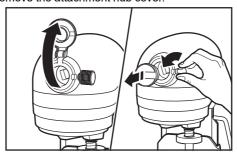
5. Insert the Main Housing into the attachment hub, make sure the power shaft fits into the square hub socket. If necessary, rotate the attachment back and forth for proper fitment. The pin on the attachment housing will fit into the notch of the hub rim when in the proper position.
