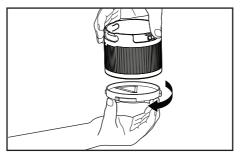
2. Insert the Ice Cup Sleeve into the Detachable Ice Cup, then insert a prepared Ice Puck. Be sure to insert the ice puck with the cross hatches facing upward.
