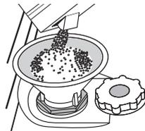
Position the funnel (see figure) and fill the salt reservoir right up to its edge (approximately 1 kg); it is not unusual for some water will spill out. Remove the funnel and wipe any salt residue away from the opening.
