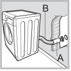
Make sure you do not push the tumble dryer too far backwards, as this could lead to the ventilation hose being crushed, bent or even disconnected. There should be no cuts, kinks or "U"-shaped bends in the hose, as these could impede ventilation or trap condensation.
