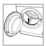
! Do not use the dryer unless the filter has been replaced in its holder.
