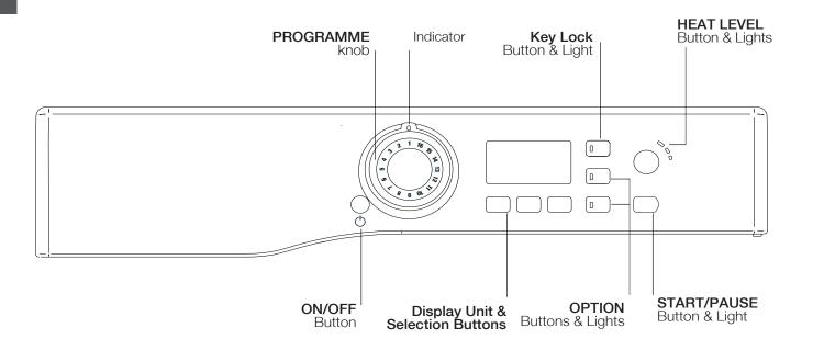
The **ON/OFF** button  $\odot$ : If the dryer is running and this button is pressed and held for more that 3 seconds the dryer is turned off, it counts down 3, 2, 1, Off and the programme is then cancelled. Press and hold for more than 3 seconds and the dryer reactivates.
