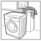
The air emitted by the tumble dryer must not be expelled in the same duct as used for the fumes produced by different appliances which burn gas or other fuels.
