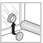
towards the air inlet pipe on the rear of the appliance. The ventilation hose must always be fitted to ensure
