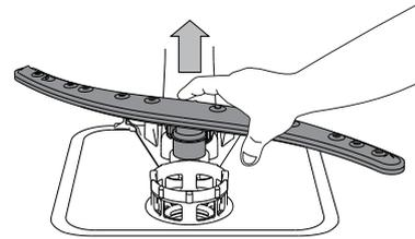
The lower spray arm may be removed by pulling it upwards.
