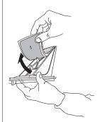
Fix the filter foam on the bottom filter. Clean the filter chamber of the dryer with a damp cloth or carefully with a vacuum cleaner. Insert the bottom filter again. Clap the filter handle down and close the bottom flap.
