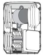
For pots, lids, plates, salad bowls, cutlery etc... Large plates and lids should ideally be placed at the sides to avoid interferences with the spray arm.
