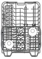
The upper rack is fitted with a sliding tray which can be used to hold small crockery and cutlery. For optimum washing performance, avoid positioning bulky crockery directly below the tray. The tray is removable.
